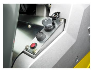
Available with crank handle or electric starter. The electric starter model is conveniently started with an ignition key.
