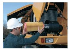
**Front Compartment.** The right front service compartment tilts providing ground level access to the batteries, ATAAC, AC condenser and the air filter.
