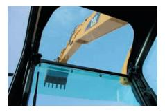
**Skylight.** A unique large polycarbonate skylight provides excellent upward visibility.
