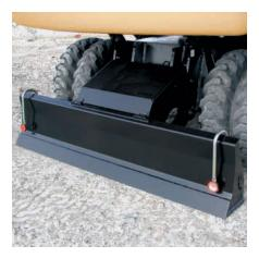
**Dozer Blade.** The pin-on design allows the dozer blade to be mounted on the front and/or rear and is used for leveling, clean-up work and for stabilizing the machine during digging applications. The large dozer bottom and parallel design provide minimized ground pressure.
