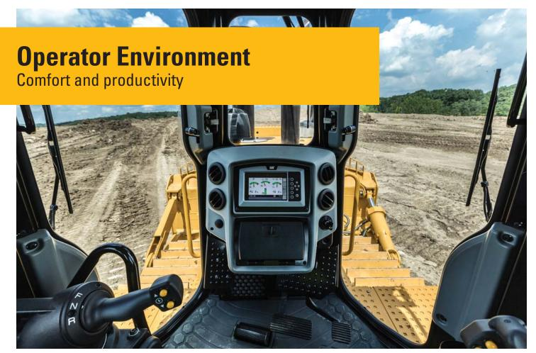
A quiet, comfortable cab, with an Integrated Roll Over Protection Structure (ROPS), gives operators greater all around visibility to enhance safety and productivity. Pressurization helps keep dust out for a cleaner operating environment. A low-effort single tiller-style handle controls direction and gear selection for ease of operation.
