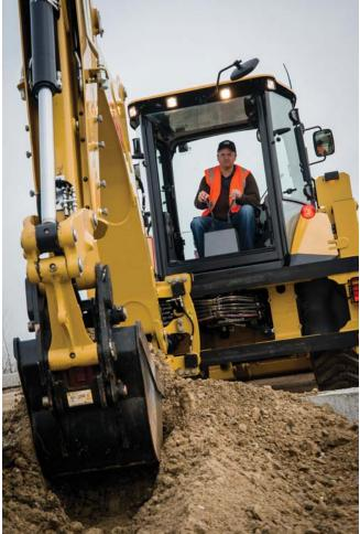
The 434F2 is fitted with mechanical controls providing low effort operation, with the ability to choose between ISO (Excavator) or SAE (Backhoe) control patterns. Providing easy and safe operation for operators of any experience or ability.
